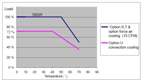
The recommended direction of the external air should be over the input terminal block, exiting over the output terminal block. The minimum recommended air volume for the correct cooling is 15CFM. If the internal fan is fitted, leave a minimum of 2" (50mm) clearance on intake and exhaust to avoid restricting airflow.
