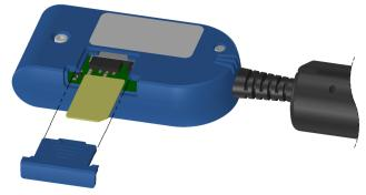
2. Insert the SIM card into the card holder with the gold contact side facing down as shown.
