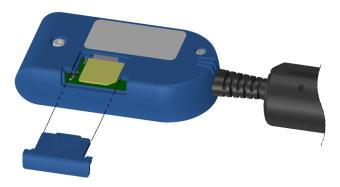
3. Verify that the SIM card fits into the holder properly and replace the cover.
