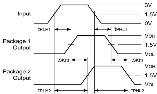
$$t_{SK(o)} = |t_{PLHy} \cdot t_{PLHx}| \text{ or } |t_{PHLy} \cdot t_{PHLx}|$$
