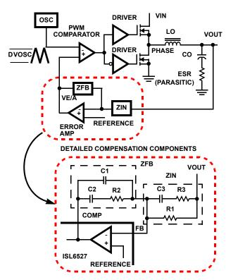
FIGURE 5. VOLTAGE-MODE BUCK CONVERTER COMPENSATION DESIGN
