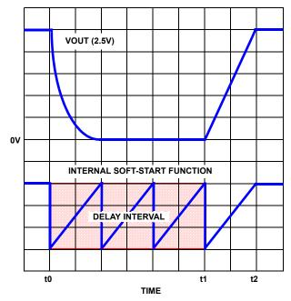
FIGURE 3. OVERCURRENT PROTECTION RESPONSE
