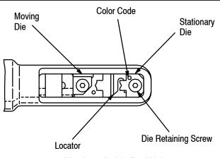
Dies Installed in Tool Yoke
