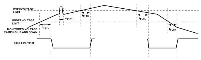
FIGURE 3. ISL8702A, ISL8703A, ISL8704A, ISL8705A FAULT OPERATIONAL DIAGRAM
