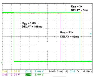
FIGURE 9. ENABLE\_X TO ENABLE\_X DISABLING
