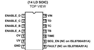
ISL8701A, ISL8703A, ISL8705A PINS 1-4 ARE ENABLE# FUNCTION ISL8704A, ISL8705A PIN 9 IS SEQ\_EN# FUNCTION
