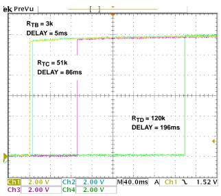
FIGURE 8. ENABLE\_X TO ENABLE\_X ENABLING
