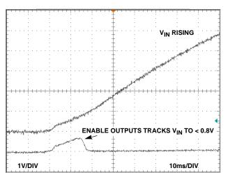
FIGURE 11. ENABLE AS VIN RISES
