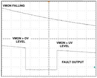
FIGURE 7. VMONITOR FALLING TO FAULT
