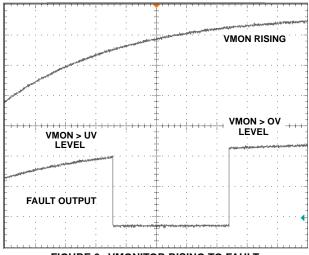
FIGURE 6. VMONITOR RISING TO FAULT
