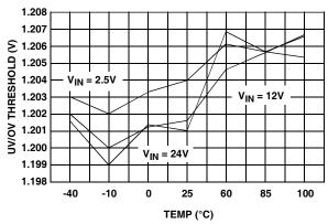
FIGURE 4. UV/OV RISING THRESHOLD
