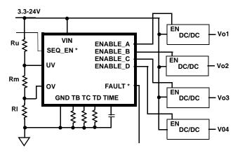
\* SEQ\_EN and FAULT are not available on ISL8700A and ISL8701A
