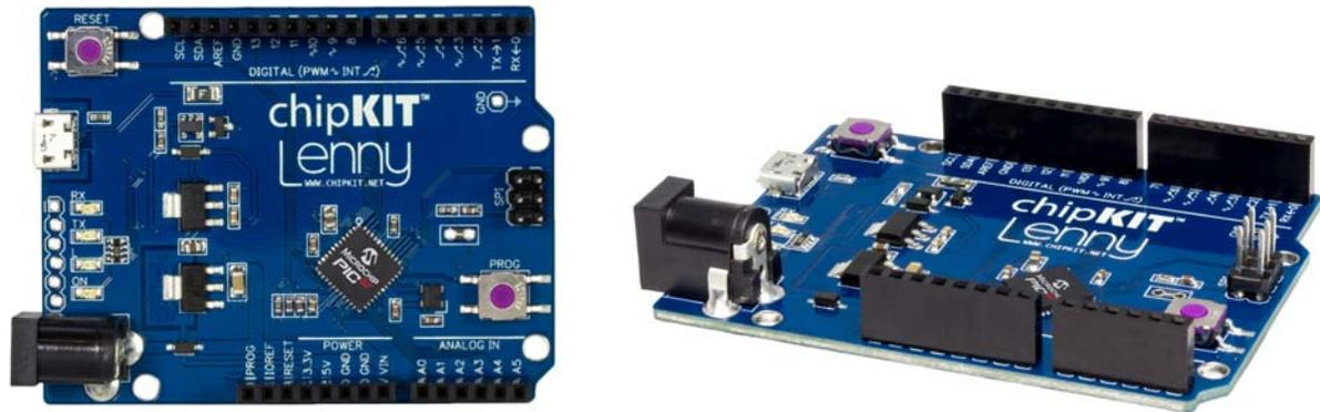
The chipKIT Lenny was inspired by the Arduino Leonardo, and adds additional capabilities afforded by its 32-bit microcontroller. The Lenny has 27 available I/O lines, 6 of which can be used as analog inputs. Based on the 32-bit PIC32MX270F256D microcontroller, operating at 3.3 volts and 40 MHz. Direct access to the USB peripheral controller enables the Lenny to emulate many types of USB devices; note that this functionality will be available in a future library.
