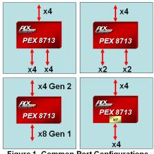
Figure 1. Common Port Configurations
