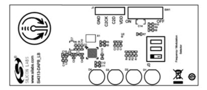
Figure 2. Si4313 LED Receiver Board Low Band with PCB Antenna (P/N 4313-DAPB\_LB)
