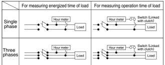
Note) Make the connection with the accompanying flat connector first and then with the hour meter's terminal (#187). In such case, be sure to cover the connection with the accompanying insulating sleeve.
