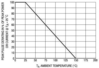
Figure 3. Steady State Power Derating Curve
