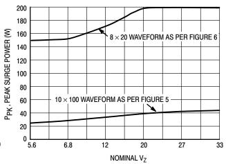
Figure 8. Typical Maximum Non-Repetitive Surge Power, P<sub>pk</sub> versus V<sub>Z</sub>
