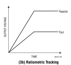
Figure 3. Two Different Modes of Output Voltage Tracking
