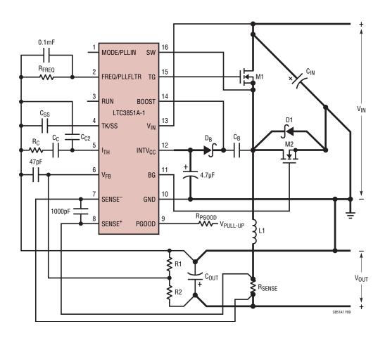
Figure 9. LTC3851A-1 Layout Diagram
