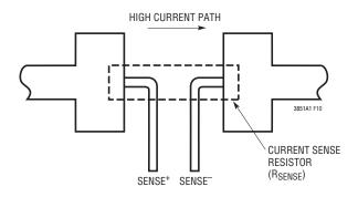
Figure 10. Kelvin Sensing R<sub>SENSE</sub>
