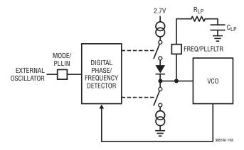
Figure 8. Phase-Locked Loop Block Diagram
