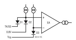
Figure 5. Equivalent Input Circuit of Error Amplifier
