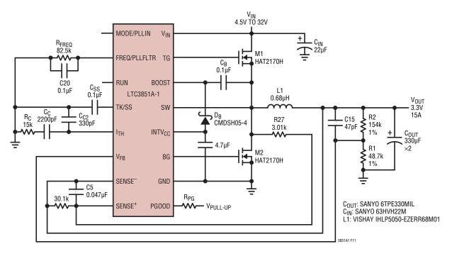
Figure 11. High Efficiency 3.3V/15A Step-Down Converter
