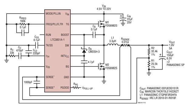
Figure 12. 1.8V/5A Converter from Design Example with Pulse Skip Operation
