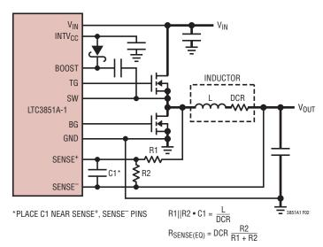
Figure 2. Current Mode Control Using the Inductor DCR
