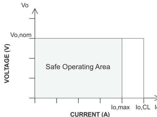
Figure 2. Maximum Output Current Safe Operating Area
