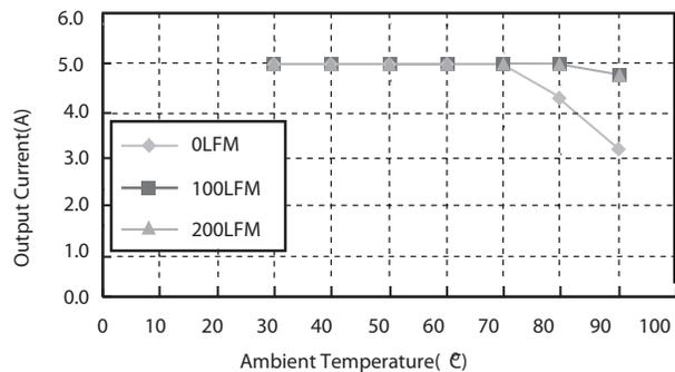
Figure 3. Typical Power De-rating for 5V IN 3.3Vout
