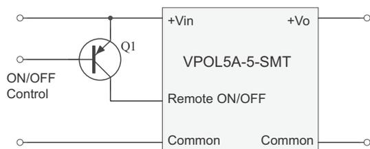
Figure 4. Negative Remote On/Off Input Drive Circuit
