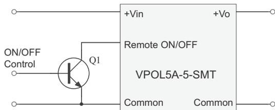
Figure 3. Positive Remote On/Off Input Drive Circuit
