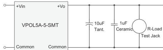
Figure 13. Output Voltage Ripple and Noise Measurement Set-Up
