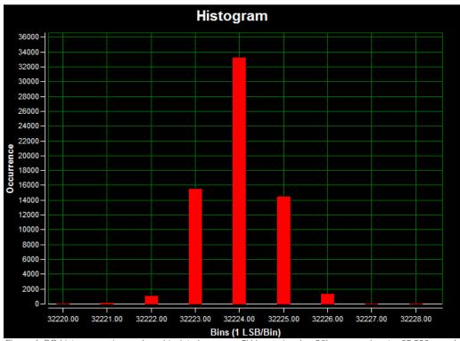
Figure 4. DC histogram using on-board isolated power; a 5V input signal; a 20ksps sample rate; 65,536 samples; a code spread of 8 LSBs with 96.3% of the codes falling within the three center LSBs; and a standard deviation of 0.785.
