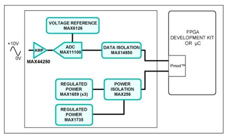
Figure 1. The Fresno subsystem design block diagram.
