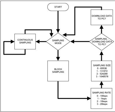
Figure 2. The Fresno firmware flowchart.
