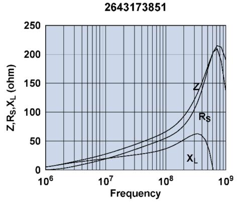
Impedance, reactance, and resistance vs. frequency.
