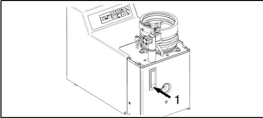
If the conductor is inserted, the CF 1000 will not start.
