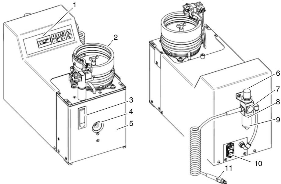
Figure 2-1 Operating components
