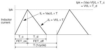
Given that the period when current flows into coil is
