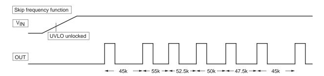
Switching frequency is changed as follows. ...  $\times 0.9 \rightarrow \times 1.1 \rightarrow \times 1.05 \rightarrow \times 1 \rightarrow \times 0.95 \rightarrow \times 0.9 \rightarrow \times 1.1 \dots$ It's repeated by this loop.
