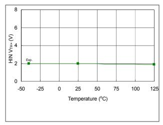
Fig. 40. HIN V<sub>TH+</sub> vs. Temperature
