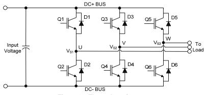
Figure 11: Three phase inverter
