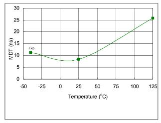
Fig. 46. Deadtime Matching vs. Temperature
