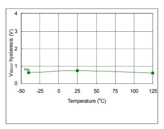
Fig. 28.  $V_{BS}$  Supply UV Hysteresis vs. Temperature
