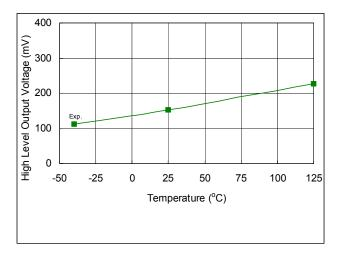
Fig. 36. High Level Output Voltage vs. Temperature
