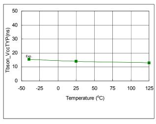
Fig. 42. Tbson\_V<sub>CC</sub>TYP vs. Temperature
