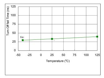
Fig. 26. Turn-off Rise Time vs. Temperature
