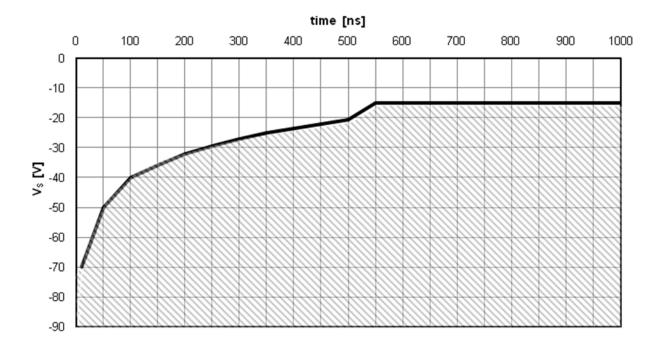
Figure 19: Negative V<sub>S</sub> transient SOA for IRS25091 @ VBS=15V
