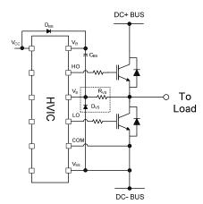
Figure 22: V<sub>S</sub> clamping diode
