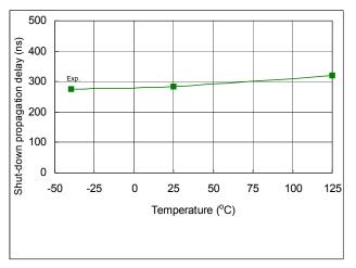
Fig. 43. Shut-down Propagation Delay vs. Temperature
