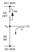
Figure 14: D3 conducting
