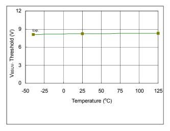
Fig. 34. V<sub>BSUV-</sub> Threshold vs. Temperature
