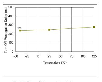
Fig. 24. Turn-off Propagation Delay vs. Temperature
