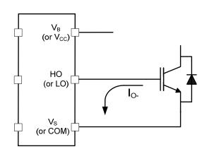
Figure 2: HVIC sinking current
