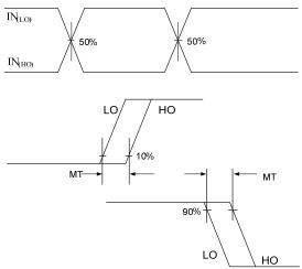
Figure 7: Delay Matching waveform Definition
