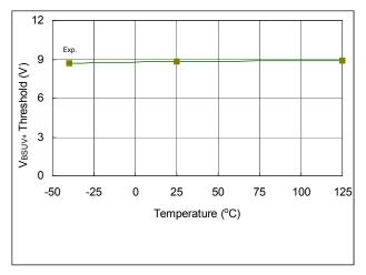
Fig. 33. V<sub>BSUV+</sub> Threshold vs. Temperature
