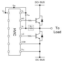
Figure 21: V<sub>S</sub> resistor
