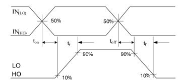
Figure 3: Switching time waveforms
