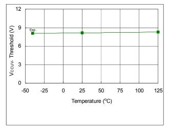
Fig. 32. V<sub>CCUV-</sub> Threshold vs. Temperature
