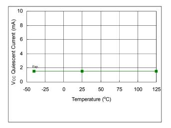
Fig. 29.  $V_{\text{CC}}$  Quiescent Supply Current vs. Temperature
