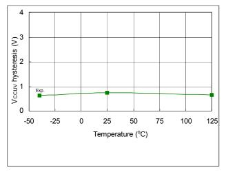
Fig. 27. V<sub>CC</sub> Supply UV Hysteresis vs. Temperature
