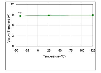
Fig. 31. V<sub>CCUV+</sub> Threshold vs. Temperature
