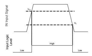
Figure 8: HIN & LIN input thresholds
