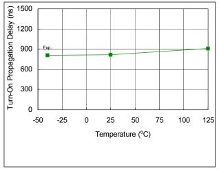
Fig. 23. Turn-on Propagation Delay vs. Temperature
