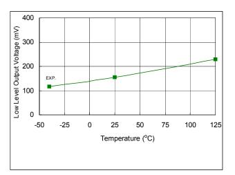
Fig. 35. Low Level Output Voltage vs. Temperature
