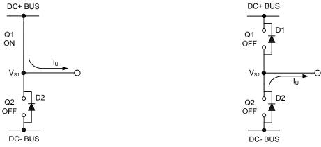
Figure 12: Q1 conducting
