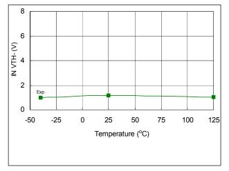
Fig. 39. LIN  $V_{\text{TH-}}$  vs. Temperature
