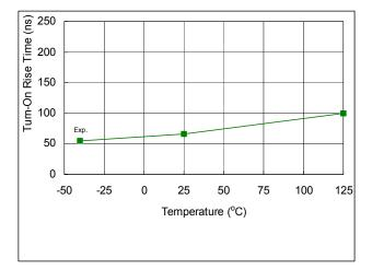
Fig. 25. Turn-on Rise Time vs. Temperature
