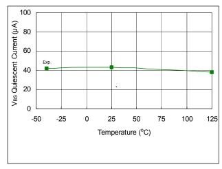
Fig. 30. V<sub>BS</sub> Quiescent Supply Current vs. Temperature
