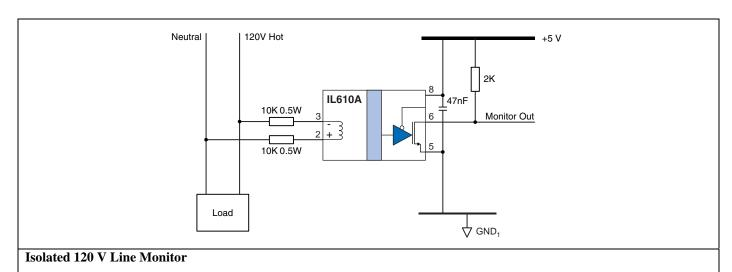
The wide input voltage range of IL600 Isolators allow connection to line voltage through current-limiting resistors. In this illustrative circuit, "Monitor Out" goes low when line voltage exceeds approximately 100 V, and high when line voltage drops below approximately 10 V.
