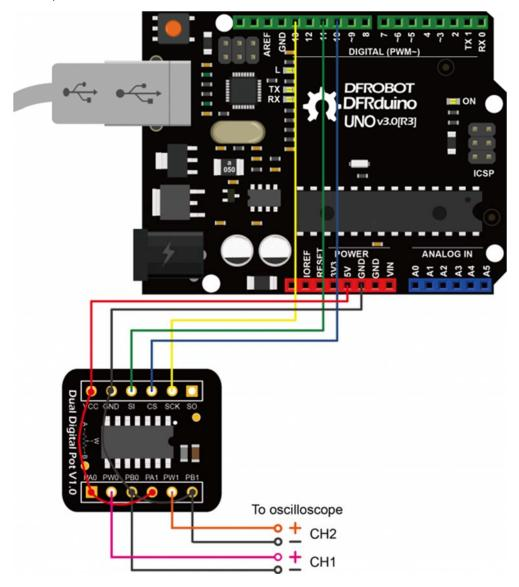
Arduino UNO Connection Diagram
