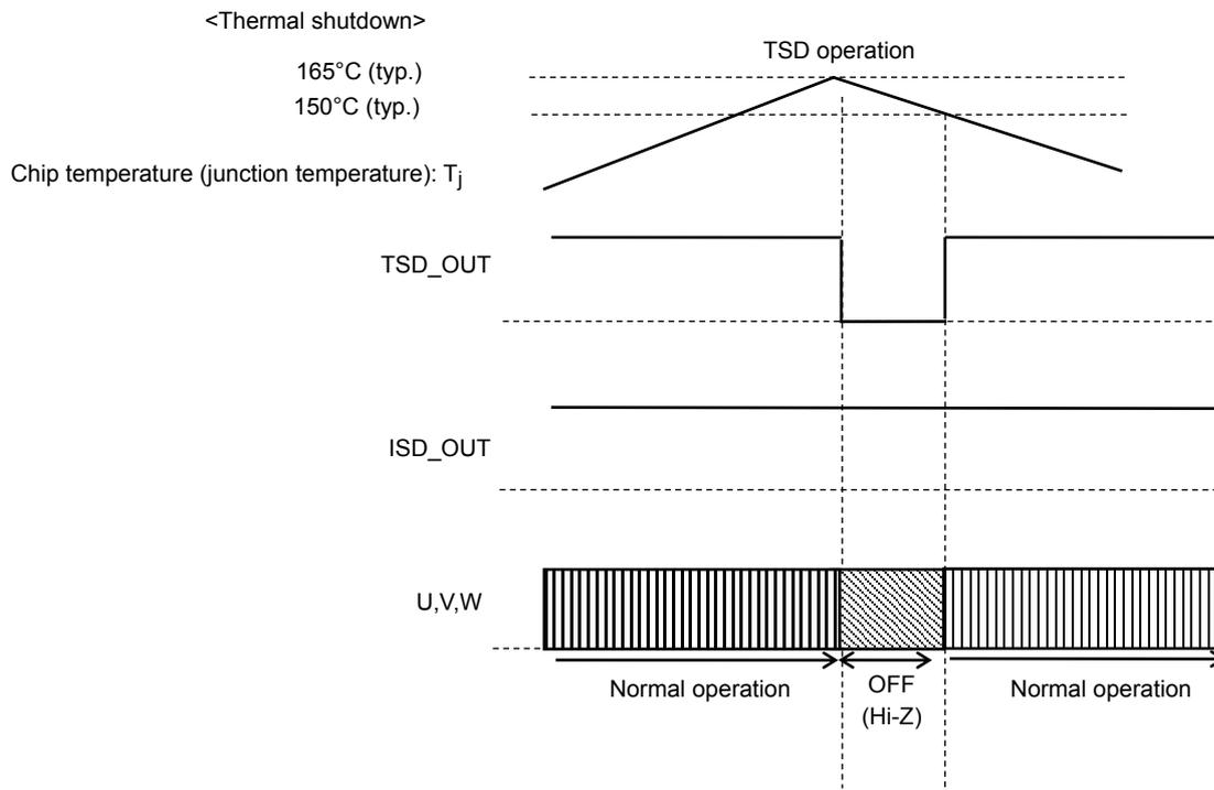
Note: The TSD circuit is activated if the absolute maximum junction temperature rating ( $T_j$ ) of 150°C is violated. Note that the circuit is provided as an auxiliary only and does not necessarily provide the IC with a perfect protection from any kind of damages.
