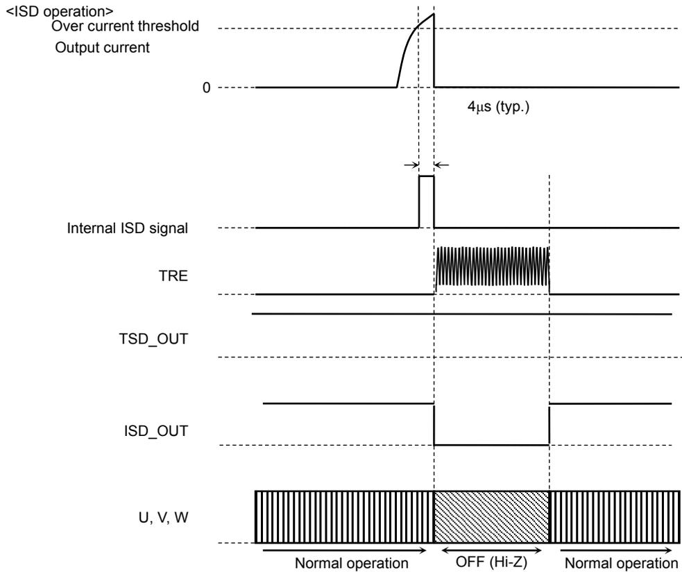
Note: The ISD circuit is activated if the absolute maximum current rating is violated. Note that the circuit is provided as an auxiliary only and does not necessarily provide the IC with a perfect protection from damages due to overcurrent caused by power fault, ground fault, load-short and the like.
