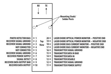
Figure 5. Pin Out Diagram (Top View)
