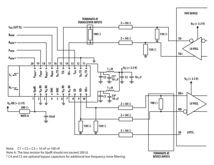
Figure 6a. Recommended dc coupled interface circuit
