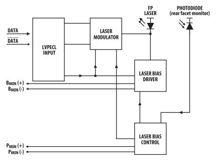
Figure 2. Simplified Transmitter Schematic
