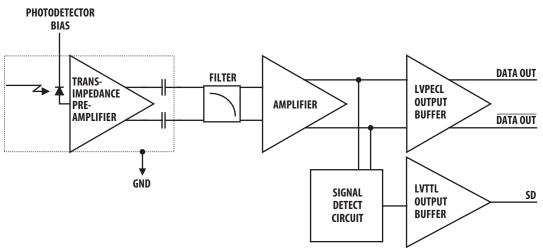
Figure 1. Receiver Block Diagram
