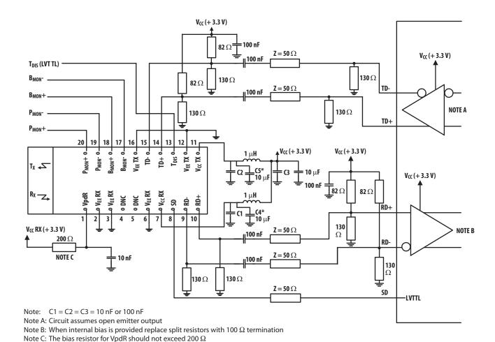
Figure 6b. Recommended ac coupled interface circuit
