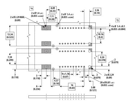
Figure 7. Recommended Board Layout Hole Pattern
