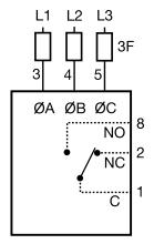
F = Fuses ØA = Phase A = L1 ØB = Phase B = L2 ØC = Phase C = L3 NO = Normally Open NC = Normally Closed
