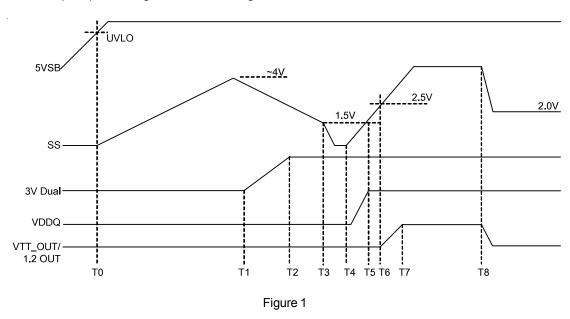
T0 to T3: After initial power-up, the IC will ignore all logic inputs for a time period (T3-T0) of about:
