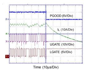
Figure 6. Over Current Protection Waveform
