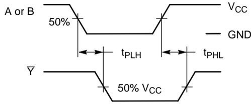
Figure 3. Switching Waveforms
