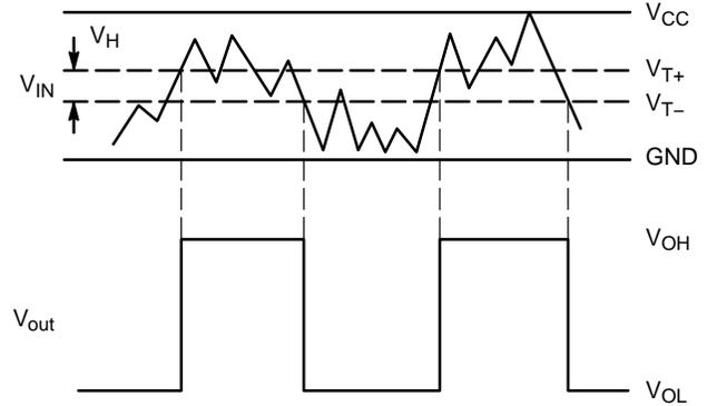
(a) A Schmitt-Trigger Squares Up Inputs With Slow Rise and Fall Times
