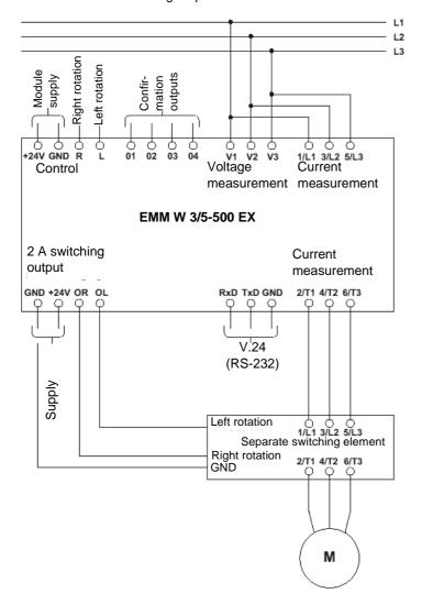
Figure 3 Connection version 1: Conductor currents < 5 A, without external current transformers
