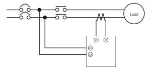
• Always turn on the control power supply for the K8AK at least 2 seconds before turning on the power for the load.
