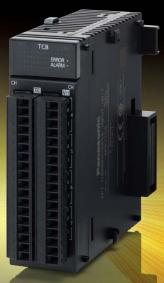
Thermocouple multiple analog input unit AFP7TC8
