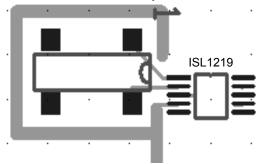
FIGURE 22. SUGGESTED LAYOUT FOR ISL1219 AND CRYSTAL
