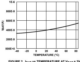
FIGURE 2.  $I_{BAT}$  vs TEMPERATURE AT  $V_{BAT}$  = 3V
