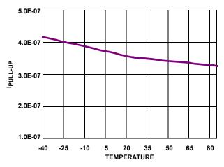
FIGURE 8. I<sub>PULL-UP</sub> vs TEMPERATURE AT V<sub>BAT</sub> = 1.8V
