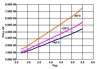
FIGURE 7. EVIN  $I_{PULL-UP}$  vs  $V_{DD}$
