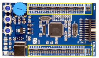
The preferred way to access the TMPM330 peripheral ports is to solder rows of pins to the prototyping grid.
