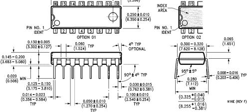
16-Lead Plastic Dual-In-Line Package (PDIP), JEDEC MS-001, 0.300" Wide Package Number N16E
