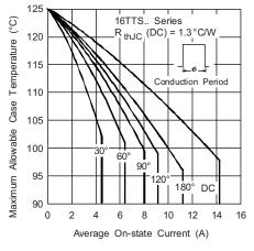
Fig. 2 - Current Rating Characteristics
