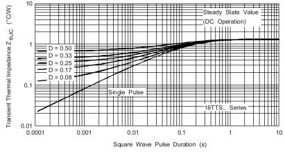
Fig. 8 - Thermal Impedance  $Z_{thJC}$  Characteristics
