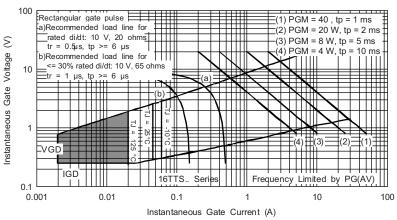
Fig. 9 - Gate Characteristics
