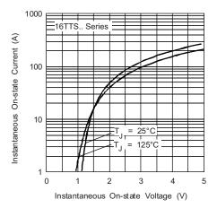
Fig. 7 - On-State Voltage Drop Characteristics
