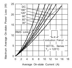
Fig. 4 - On-State Power Loss Characteristics
