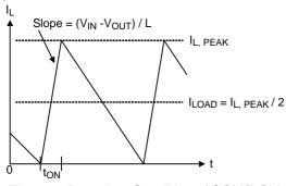
Figure 1. Boundary Condition of CCM/DCM
