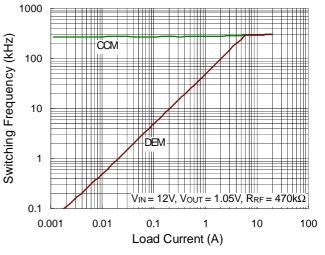
Switching Frequency vs. Load Current
