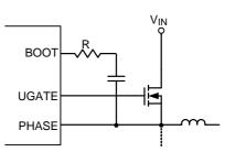
Figure 3. Reducing the UGATE Rise Time
