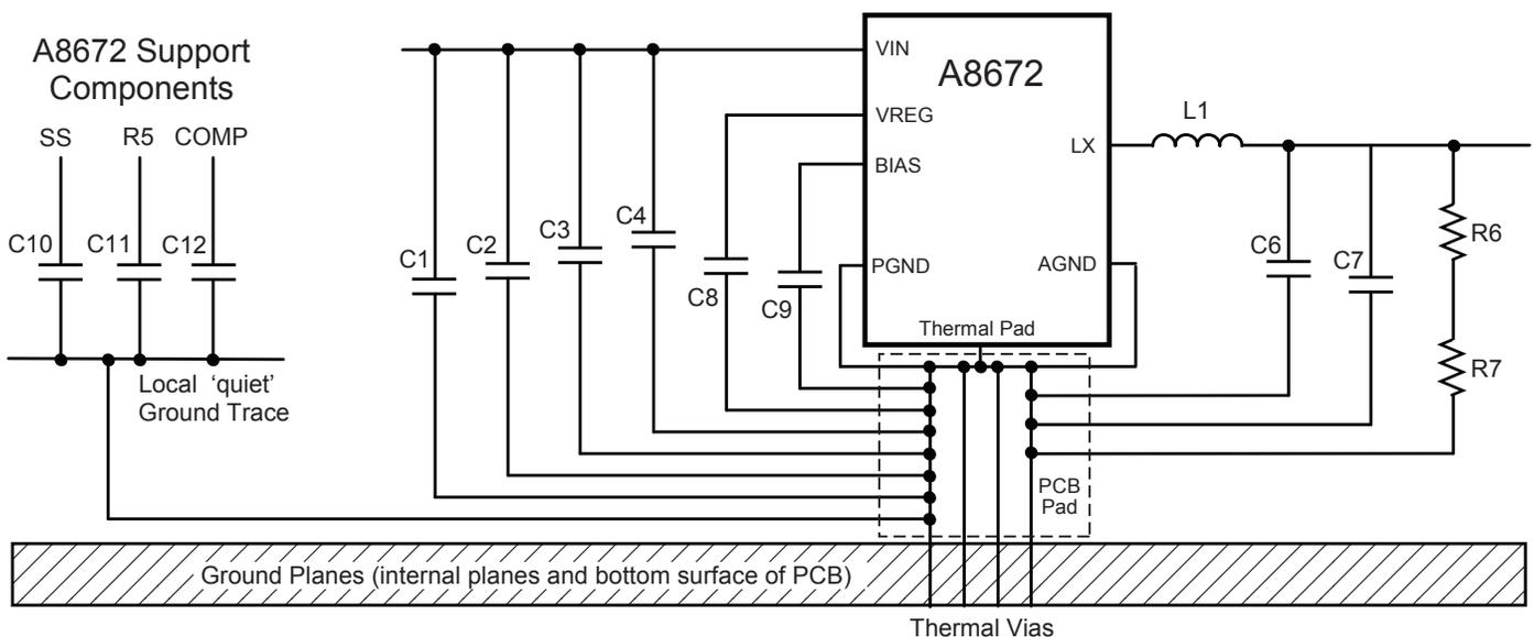
Figure 8: Layout Considerations for Mounting the A8672
