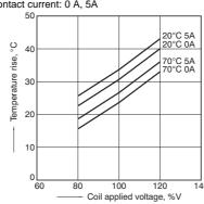
3. Ambient temperature characteristics and coil applied voltage
