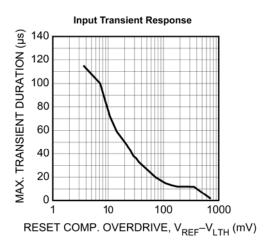
Figure 2. Input Transient Response
