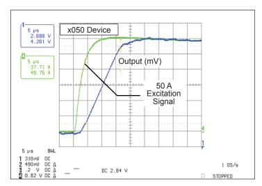
Step Response No external filter, T<sub>A</sub>=25°C
