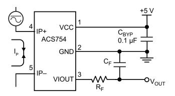
Application 1. The ACS754 outputs an analog signal,  $V_{OUT}$ . that varies linearly with the uni- or bi-directional AC or DC primary sensed current,  $I_P$ , within the range specified.  $C_F$ is recommended for noise management, with values that depend on the application.
