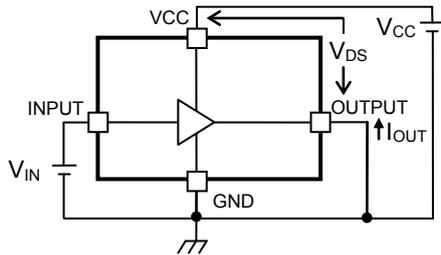
Test circuits may be omitted partially or simplified for explanatory purpose.
