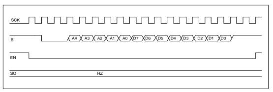
Figure 7: Write sequence into configuration register
