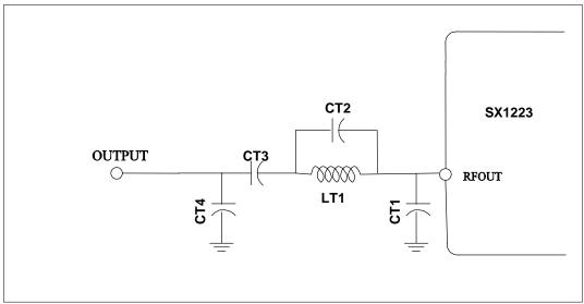
Figure 9: Transmitter output network
