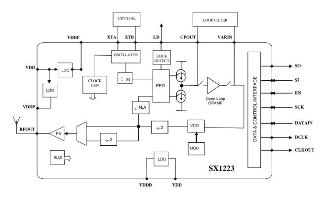
Figure 1: SX1223 block diagram
