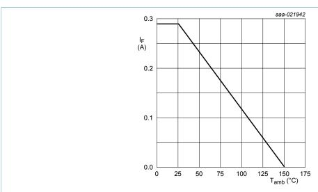
Fig. 2. Forward current as a function of ambient temperature; derating curve
