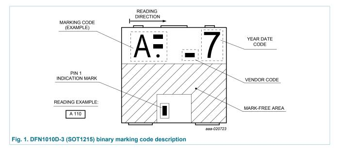
Single high-speed switching diode
