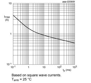
Fig. 8. Non-repetitive forward current as a function of pulse duration; maximum values
