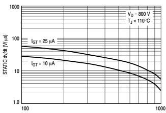
R<sub>GK</sub>, GATE-CATHODE RESISTANCE (OHMS)
