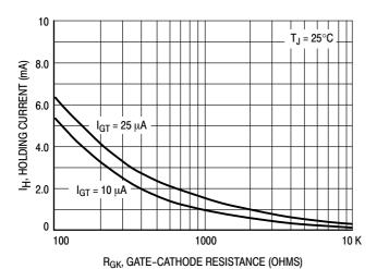
Figure 9. Holding Current versus
