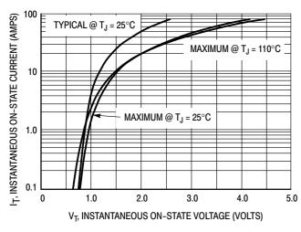
Figure 3. On-State Characteristics
