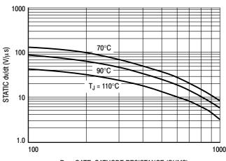
R<sub>GK</sub>, GATE-CATHODE RESISTANCE (OHMS)
