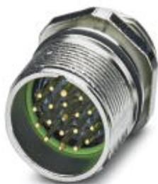
Device connector for front wall, straight, shielded: yes, SPEEDCON locking, M23, No. of pos.: 16+2+PE, type of contact: Pin, Crimp connection, Axial seal, Central fastening Pg13,5
