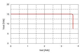
Fig. 17: Output voltage vs. load current showing current limit point and converter shutdown point. Input voltage has almost no effect on current limit characteristic.
