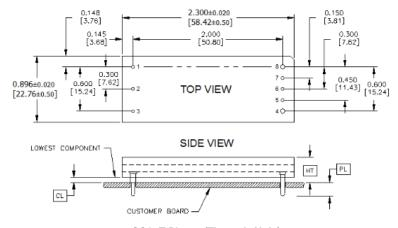
SQ24T Pinout (Through-Hole)
