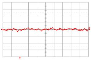
Fig. 16: Input reflected ripple current, is (10 mA/div.), measured through 10 μH at the source at full rated load current and Vin = 24 V. Refer to Fig. 14 for test setup. Time scale: 1 μs/div.
