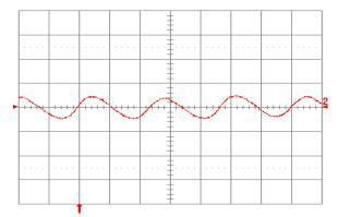
Fig. 15: Input reflected ripple current, ic (100 mA/div.), measured at input terminals at full rated load current and Vin = 24 V. Refer to Fig. 14 for test setup. Time scale: 1 μs/div.
