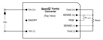
Figure C. Configuration for increasing output voltage.
