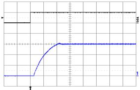
Fig. 9: Turn-on transient at full rated load current (resistive) with no output capacitor at Vin = 24 V, triggered via ON/OFF pin. Top trace: ON/OFF signal (5 V/div.). Bottom trace: output voltage (5 V/div.). Time scale: 1 ms/div.
