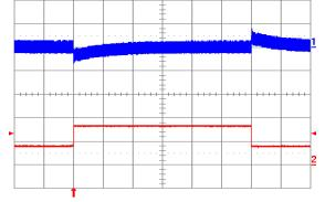
Fig. 11: Output voltage response to load current step-change (0.825 A – 1.65 A – 0.825 A) at Vin = 24 V. Top trace: output voltage (200 mV/div.). Bottom trace: load current (1 A/div.). Current slew rate: 0.1 A/μs. Co = 1 μF ceramic. Time scale: 0.5 ms/div.
