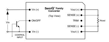
Figure A. Circuit configuration for ON/OFF function.
