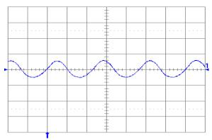
Fig. 13: Output voltage ripple (100 mV/div.) at full rated load current into a resistive load with Co = 10 μF tantalum + 1uF ceramic and Vin = 24 V. Time scale: 1 μs/div.
