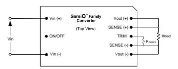
Figure D. Configuration for decreasing output voltage.
