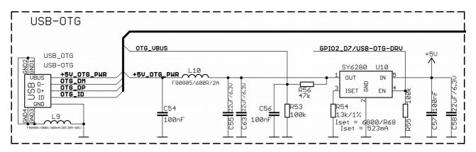
The USB\_OTG features Low Loss Power Distribution Switch SY6280 which protects the board in case the devices you have plugged to the USB\_OTG attempt to draw more current than 523mA
