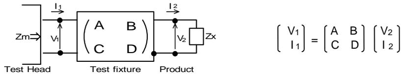
(2) The impedance of chip coil Zx and measured value Zm can be described by input/output current/voltage.
