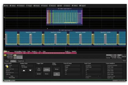
Trigger on every aspect of the FlexRay Frame as well as Symbols and Errors including FSS, BSS, FES, CRC, CID, CAS/MTS and Wakeup by selecting the appropriate boxes.
