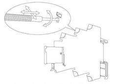
Do not insert two or more wires in the hole. Wires may come in contact with the spring causing a temperature rise or be subject to sparks.
