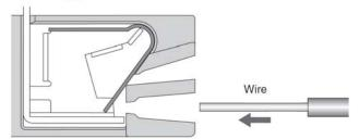
Insert the exposed conductor into the connection hole.
