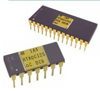
The HTADC12 is a high temperature, single supply, 12-bit, 100kSPS, analog-to-digital converter with on-chip buffered voltage reference and an on-chip analog input buffer. The HTADC12 uses a Successive Approximation Register (SAR) architecture that does not require an input sample-and-hold amplifier to provide 12-bit resolution at 100 kSPS data rates
