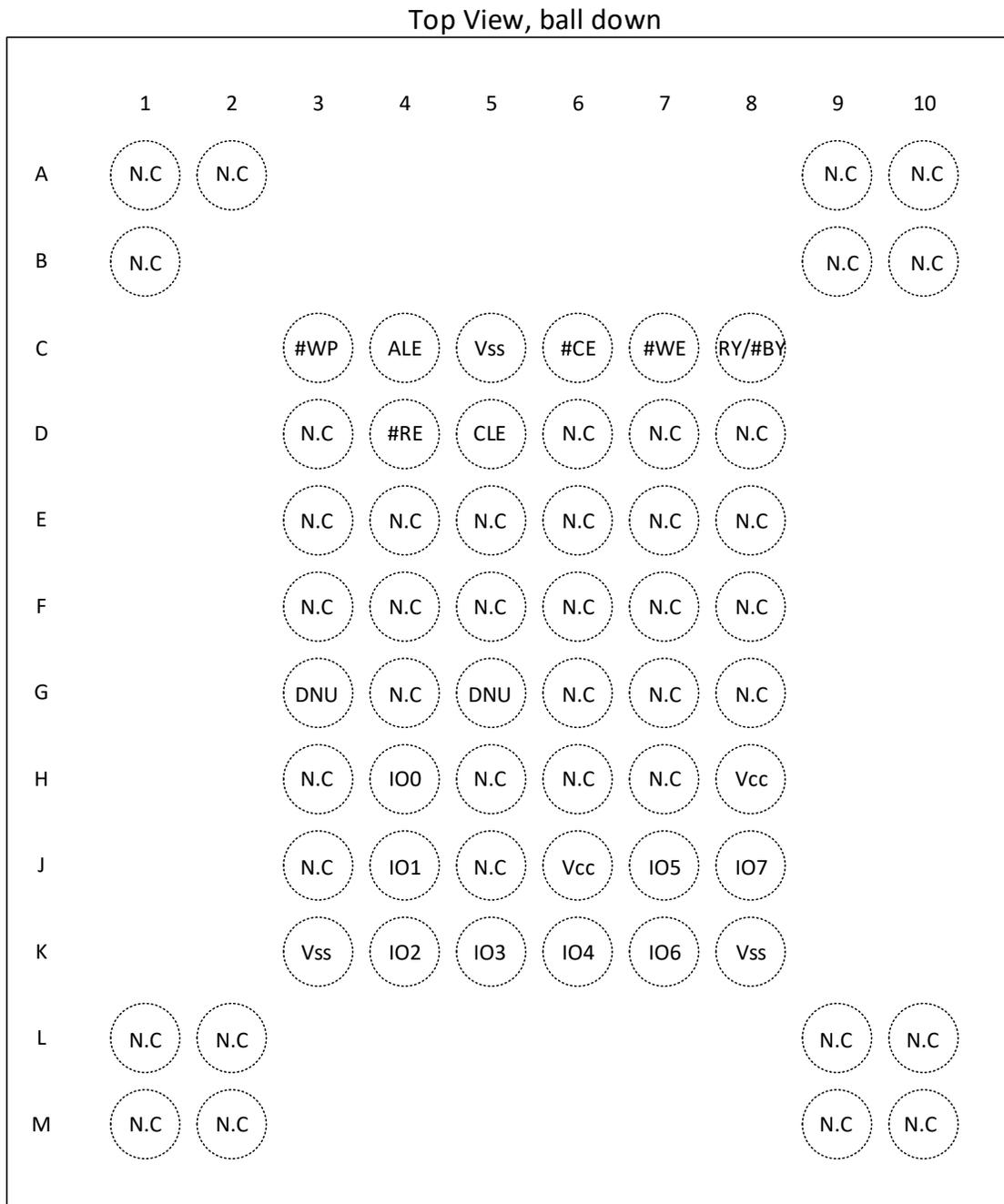
Figure 3-2 Pin Assignment 63-ball VFBGA (Package code B)
