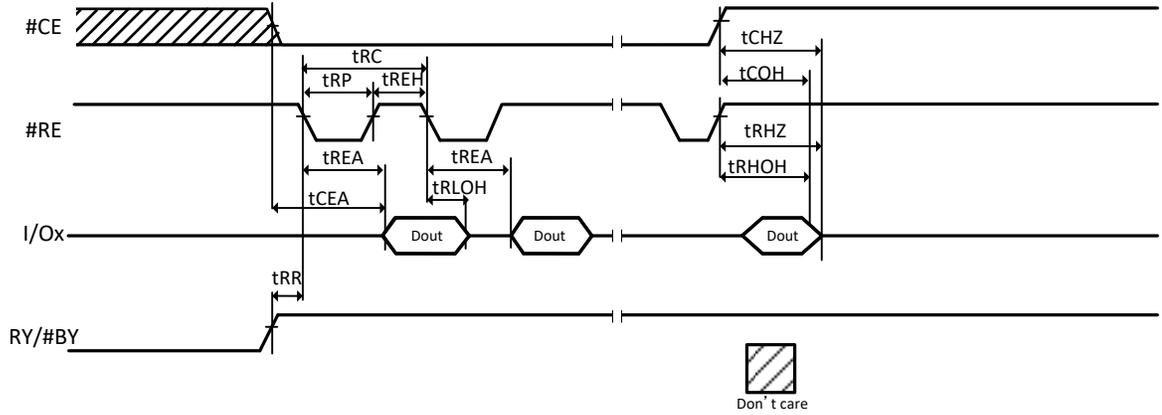
Figure 11-5 Serial Access Cycle after Read (EDO)
