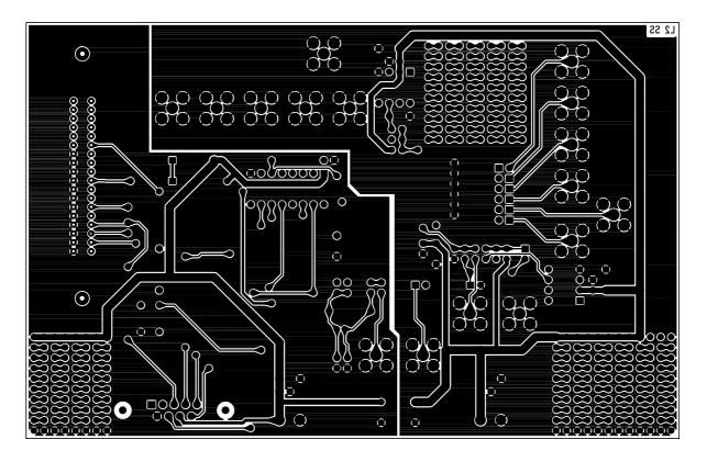
Fig. 20. The Evaluation Board Solder Side Artwork
