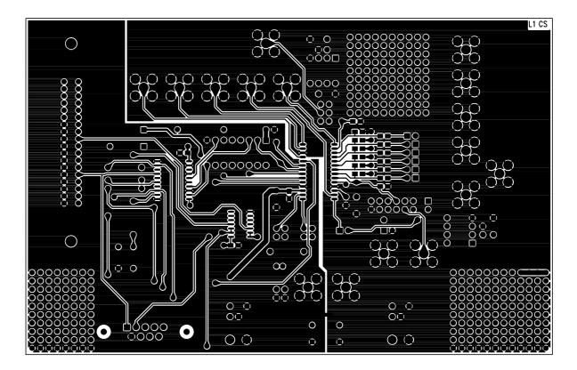
Fig. 19. The Evaluation Board Component Side Artwork
