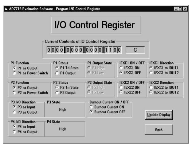
Fig. 9. The I/O and Current Source Control RegisterScreen
